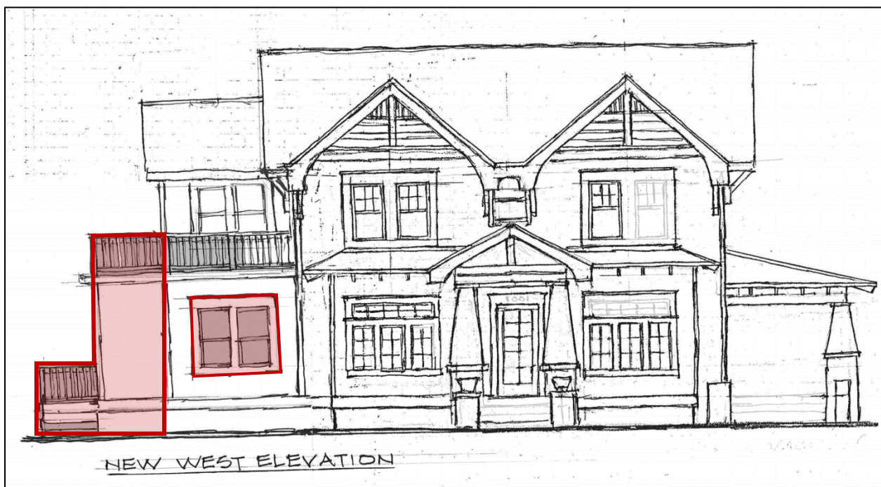
Figure 2: Proposed west elevation. The two windows to be replaced are highlighted in red.
